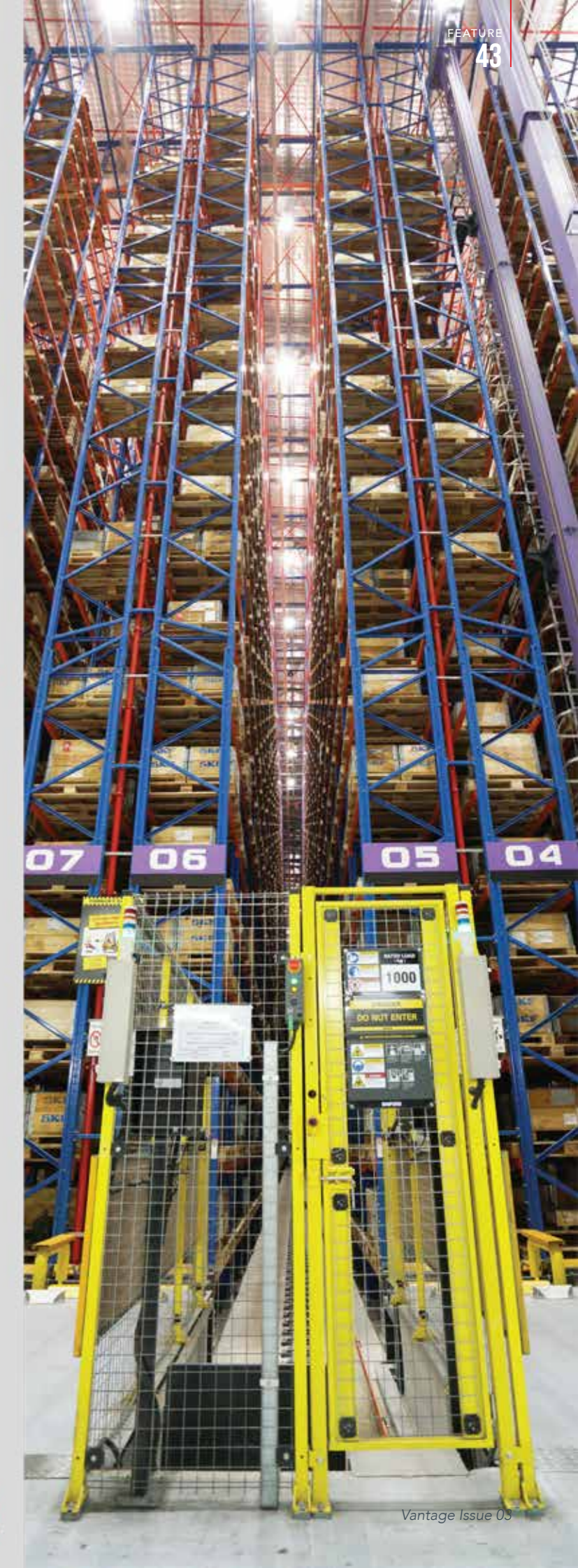
Automated Storage and Retrieval System (ASRS) for greater accuracy and improved handling ability
